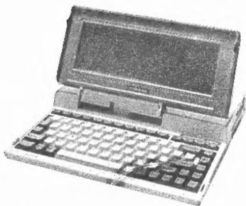
T 1000 Processador 80c88, 4.77 MHz 512 Kb RAM, 1 Floppy 3,5" 720 kb Display LCD Supertwist, Peso 2.9 kg.
